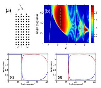
Fig. 1. (a) Geometry of the PhC grating (L=2a). (b)  $r_{-1}$  in the  $(kL,\,\theta)$ -plane at d/a=0.45 and  $\varepsilon_r=9.61$ . Dashed line, angle-independent regime of  $r_{-1}\approx 1$ ; dotted lines, approximate boundary of the stop band in which  $r_0\approx 1$ . (c), (d)  $r_0$  (solid line),  $r_{-1}$  (dashed line), and  $R=r_0+r_{-1}$  (dotted line) versus  $\theta$  at (c) kL=4.3 and (d) kL=4.4.
