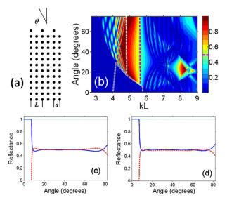
Fig. 2. (a) Geometry of the PhC grating (L=2a); (b)  $r_{-1}$  in the  $(kL,\;\theta)$ -plane at d/a=0.4 and  $\varepsilon_r=5.8$ , dashed line–angle independent regime of  $r_0\approx r_{-1}\approx 0.5$ , dashed–dotted line–angle independent regime of  $r_{-1}\approx 1$ , dotted line–approximate boundary of the stop band with  $r_0\approx 1$ , and (c), (d)  $r_0$  (solid line),  $r_{-1}$  (dashed line), and R (dotted line) versus  $\theta$  at (c) kL=5.57 and (d) kL=5.58.
