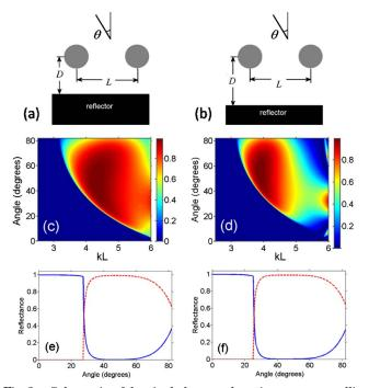
Fig. 3. Schematic of the single-layer rod grating over a metallic slab (L=2a) at (a) D=0.775a and (b) D=a;  $r_{-1}$  in the (kL,  $\theta$ )-plane (c) for configuration in case (a), and (d) for configuration in case (b), at d/a=0.45 and  $\varepsilon_r=9.61$ ; and (e), (f)  $r_0$  (solid line) and  $r_{-1}$  (dashed line) versus  $\theta$  for case (c), at (e) kL=4.3 and (f) kL=4.4.
