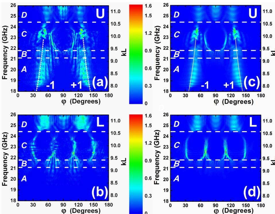
FIG. 3. Maps of the measured transmitted electric field intensity for (a) *U*-case and (b) *L*-case, and the calculated intensity at the Gaussian-beam illumination for (c) *U*-case and (d) *L*-case; TM polarization; white dashed lines show the approximate boundaries between ranges A, B, C, and D; white dotted lines show  $\varphi = \varphi_g = \pi/2 + \phi_{\pm 1}$  obtained using the grating formula.
