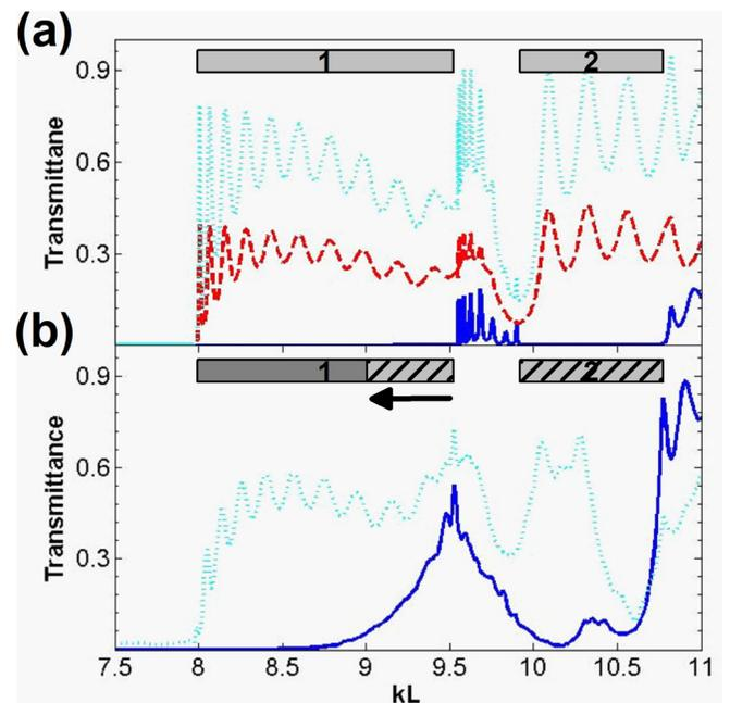
FIG. 2. Transmittance (TM polarization) as a function of  $kL$  at (a) plane-wave illumination: solid dark blue line— $t_0$ , dashed red line— $t_{\pm 1}$ , dotted cyan line— $T^{\pm}$ ; gray rectangles labeled as “1” and “2”—first and second ranges of unidirectional splitting; (b) Gaussian illumination: dotted cyan line— $T^{\pm}$ , solid dark blue line— $T^{\pm}$ ; the shaded regions in gray rectangles show the vanishing unidirectionality.
