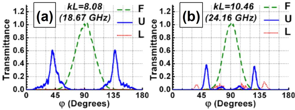
FIG. 4. The transmitted electric field intensity vs  $\varphi$  at  $kL = 8.08$  (a) and  $10.46$  (b); solid dark blue line— $U$ -case, dotted red line— $L$ -case, dashed green line—free-space case (labeled as  $F$ ); TM polarization.
