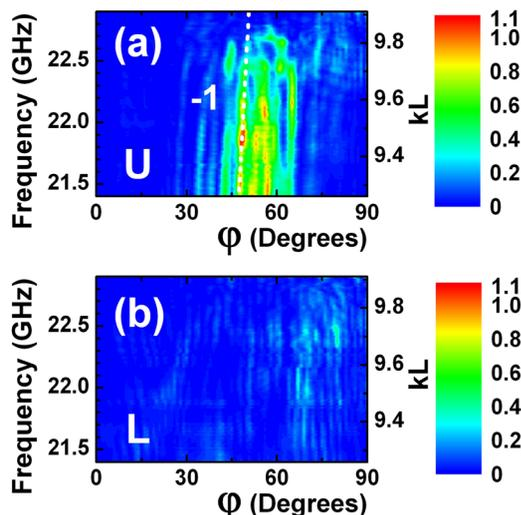
FIG. 5. The maps of the transmitted electric field intensity in  $U$ -case (a) and  $L$ -case (b); TE polarization; the white dotted line in plot (a) corresponds to  $\varphi = \varphi_g = \pi/2 + \phi_{-1}$  obtained by using the grating formula.
