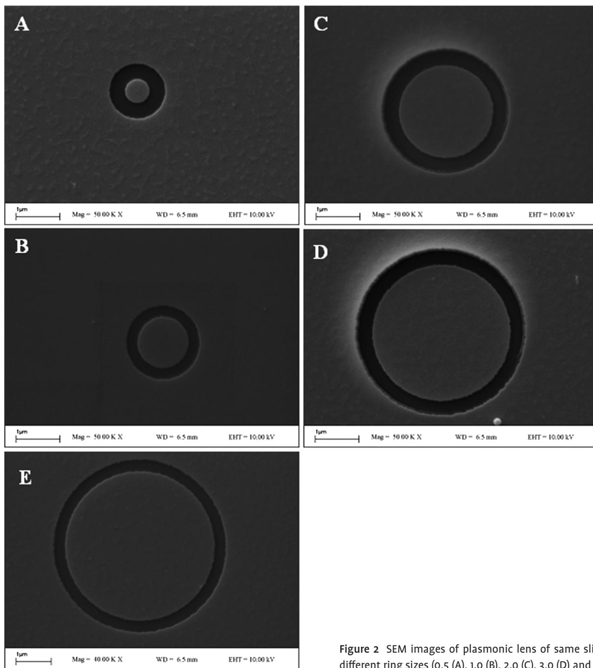
Figure 2 SEM images of plasmonic lens of same slit width with different ring sizes (0.5 (A), 1.0 (B), 2.0 (C), 3.0 (D) and 4.0  $\mu\text{m}$  (E).
