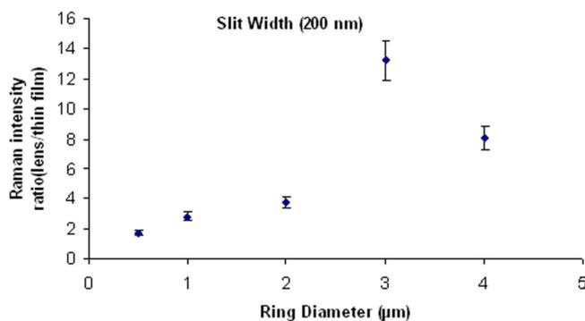
**Figure 8** SERS intensity ratio depending on ring-diameter changes.
