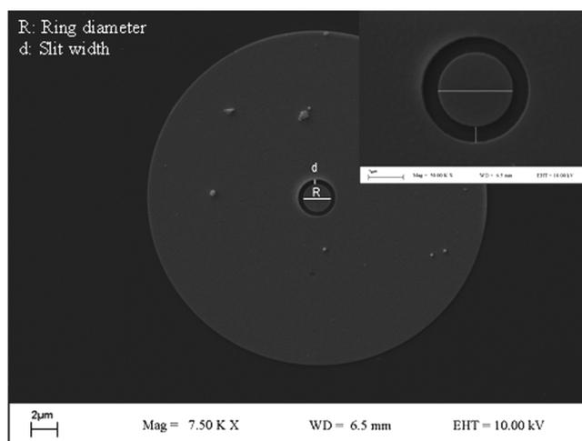
Figure 1 SEM image of ring-shaped hole on silver film.
