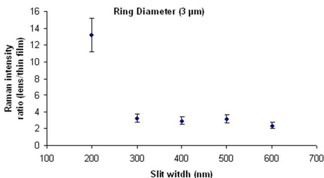
Figure 6 SERS intensity ratio depending on slit-width changes.
