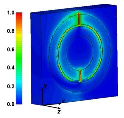
FIG. 7. (Color online) Simulated electric field intensity profile at the magnetic resonance frequency of the split ring resonator.
