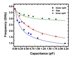
FIG. 6. (Color online) Magnetic resonance frequency of a split ring resonator as a function of loaded capacitances at different capacitive regions. The solid lines are the results obtained from the numerical models.
